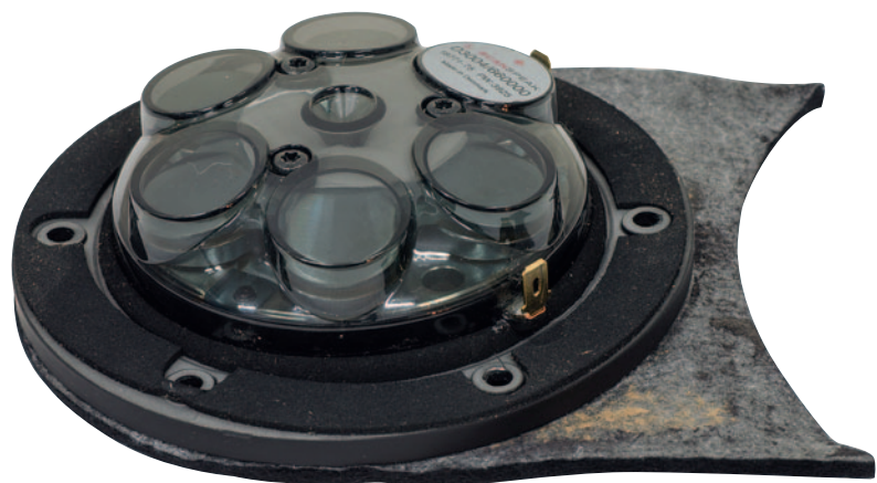
The tweeter employs a highly distinctive motor assembly, consisting of six neodymium magnet segments whose arrangement creates a small acoustic chamber, visible through the semi-transparent cover and filled with damping material.
